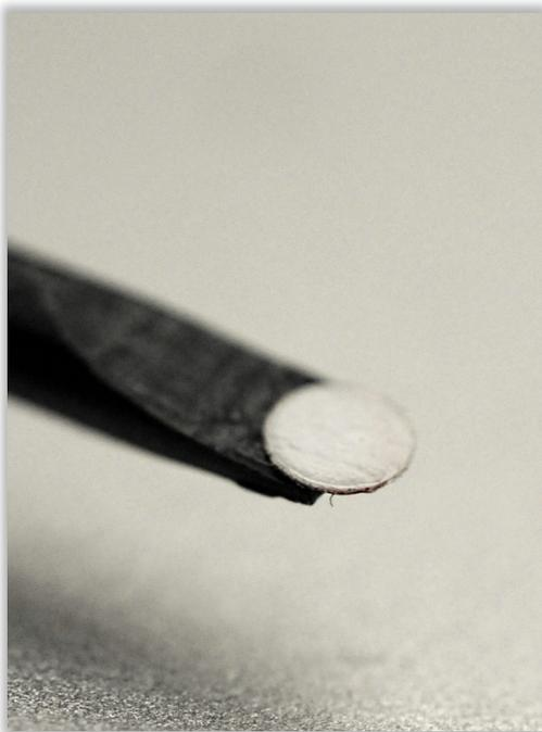
Water contact indicators such as this were placed through each phone. Upon contact with water the indicators turn red.
